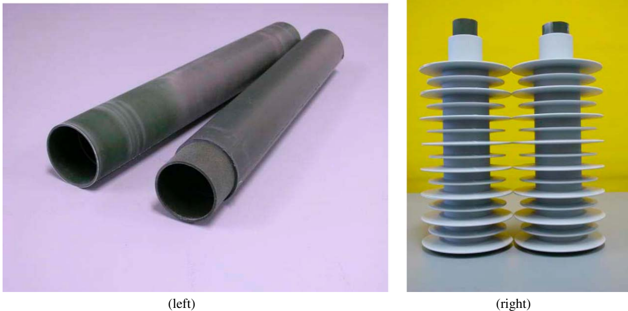
Fig. 5. Prototype of a new high voltage cable termination for \geq 84 kV (right). The inner most layer (left) provides the field grading and consists of a microvaristor composite with silicone as a flexible matrix. This field grading tube is molded into a insulating silicone housing.
